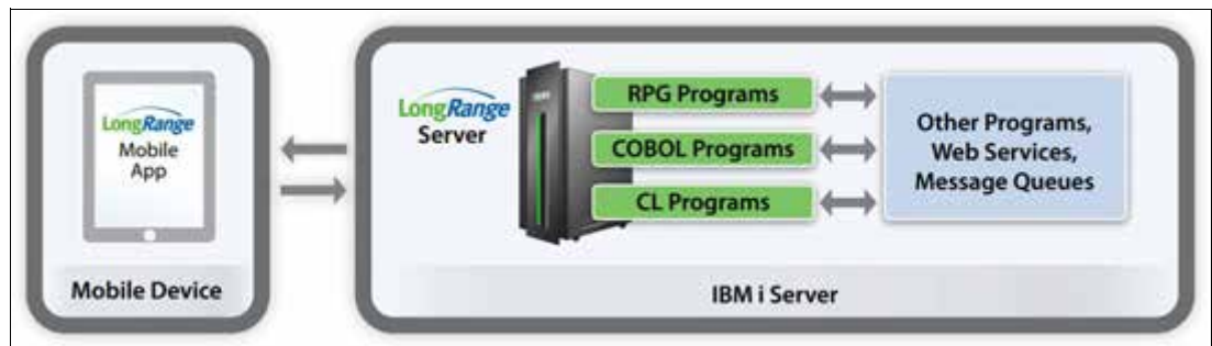
Figure 1-98 How LongRange works
